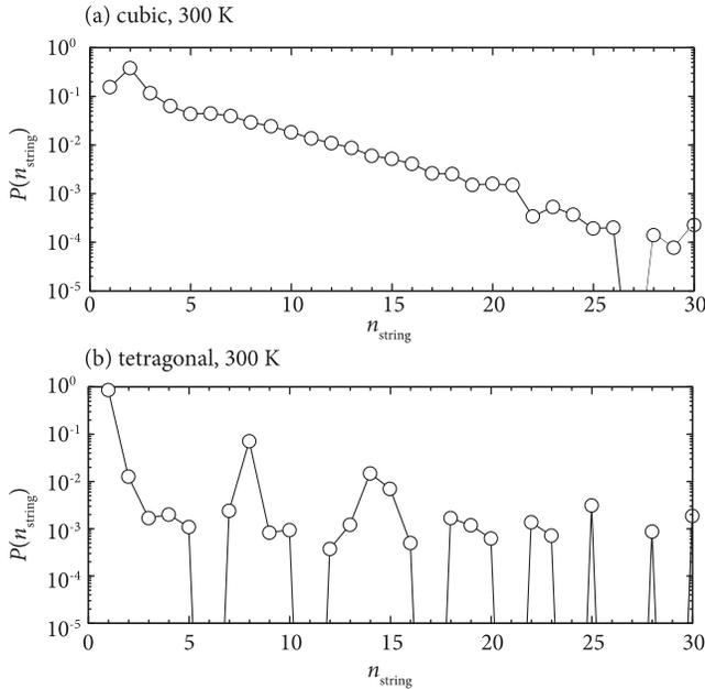
FIG. 4. Probability distribution  $P(n_{\text{string}})$  of ions contributing to strings of length  $n$  [54], for c-LLZO (upper) and t-LLZO (lower).  $\Delta t_s = 30$  ps, for consistency with the  $t_a$  value used in our excitation analysis.
