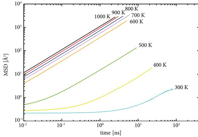
FIG. 2. Calculated mean-squared displacements (MSD) for LLZO at 300–1000 K. On a log-log plot, the diffusive regime corresponds to the sloping linear portion.
